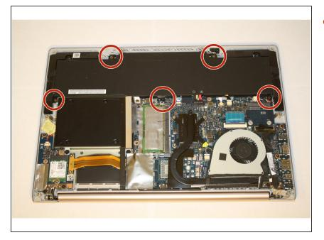
Remove the five screws attaching the battery pack by using a PH-1 screwdriver.
