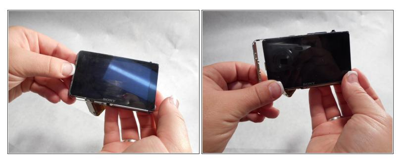
• Gently slide the LCD screen using very light pressure to the right until it pops open.
