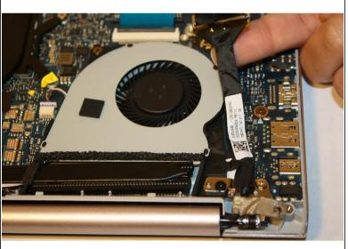
Remove the LVDS cable next to the cooling fan.
