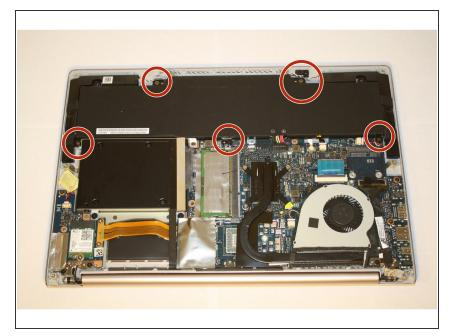
Remove the five screws from the battery pack using a PH-1 screwdriver.
