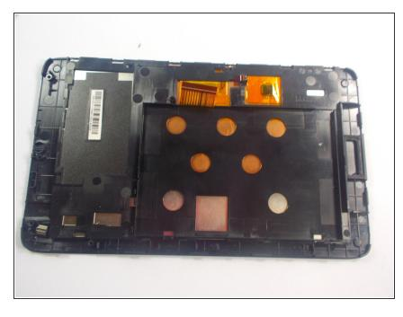
With the logic board removed the old screen is all that remains. Reassemble using a new screen as the base. To reassemble your device, follow these instructions in reverse order.
