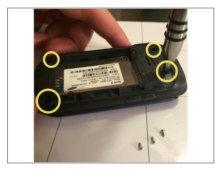
• Remove the four screws on the corners of the casing.
