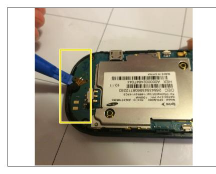
Use the plastic opening tool to pry the logic board out of the phone case from the bottom area of the phone.
