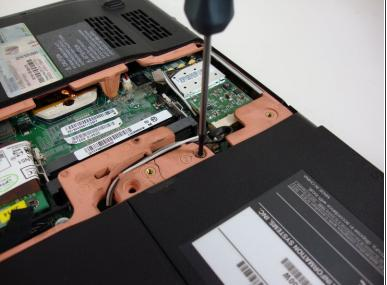
Locate and remove the circled screw with a Phillips #0 screwdriver.
