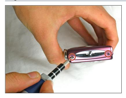
• Remove the two 2.8 mm screws on the left side of the camera.
