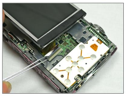
Use the <u>tweezers</u> to lift the ZIF connector which is holding the ribbon cables that connect the LCD screen to the motherboard.
