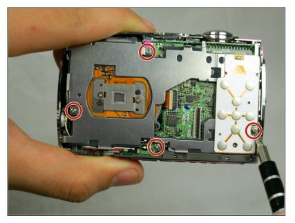
Remove the four 3.8 mm screws located near the bottom right and top left of the LCD base plate.
