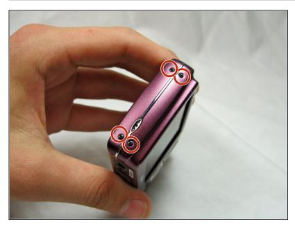
• Remove the four 2.8 mm screws on the right side of the camera.
