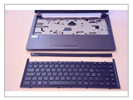
Once the cable is released, lift the keyboard out of its slot.
