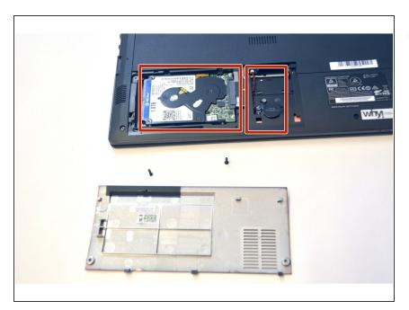
The components HDD hard disk and BIOS battery are now visible.
