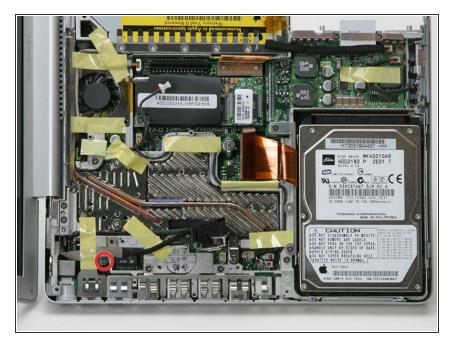
Remove the Phillips screw securing the RJ-11 Board.
