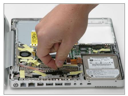
Use the black plastic pull tab to disconnect the display data cable from the logic board.
