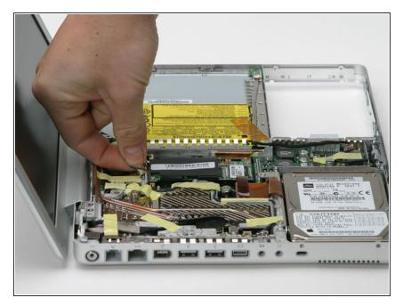
Disconnect the modem cable from the screen side of the modem and deroute it from the metal framework.
