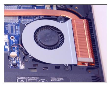
• Remove the 3 mounting screws of the fan.
