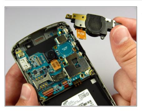
Lift the speaker out of its compartment.
