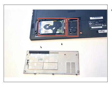
The components HDD hard disk and BIOS battery are now visible.
