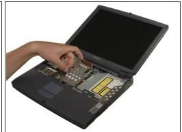
Remove the four 4mm Phillips screws around the hard drive cage.
