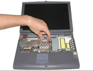
Remove the two 4mm Phillips screws in the center of the computer located on each side of the copper electrical strip.
