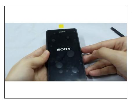
Test if the new screen works properly.
