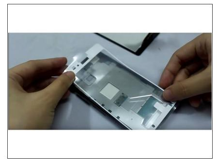
If the screen works, remove the new screen and add the double sided tape
