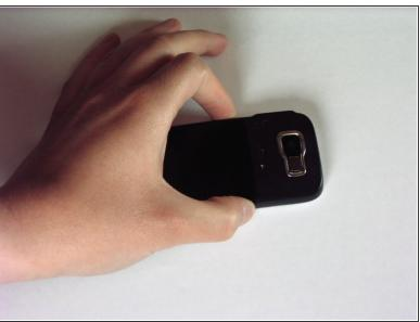
Press each release button on either side of the battery cover and simultaneously remove the battery cover from the phone.
