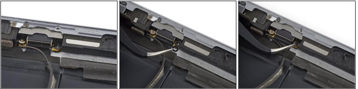
ⓘ The screw through the Lightning connector has a small washer resting on the speaker contacts. Be sure not to misplace it.
