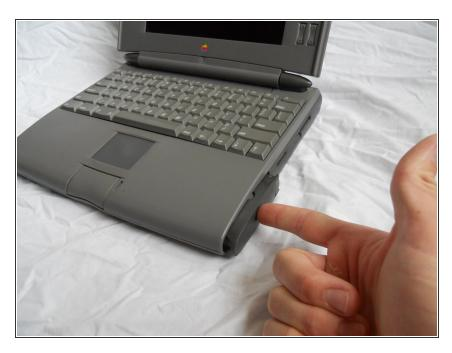
Insert new battery into battery slot.
