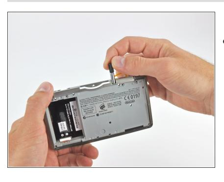
Remove the stylus from the lower case.
