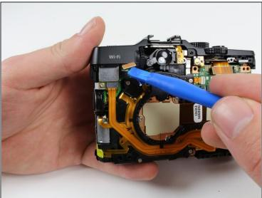
• Disconnect the cable on the back of the camera to the left of the viewfinder by lifting it up vertically using a plastic opening tool.
