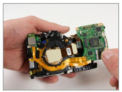
• Lift the motherboard out of the camera.
