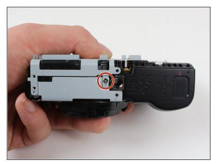
Remove the 2.7 mm screw from the bottom of the camera using a Phillips #00 screwdriver.
