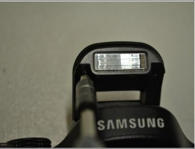
Once the flash head is up, unscrew the two black 4mm Phillips head screws located on either side of the flash bulb.
