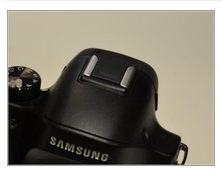
Once the screws have been removed, push the flash head back down.
