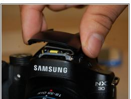
After closing the flash head, pull the black flash head cover up and off of the flash head.
