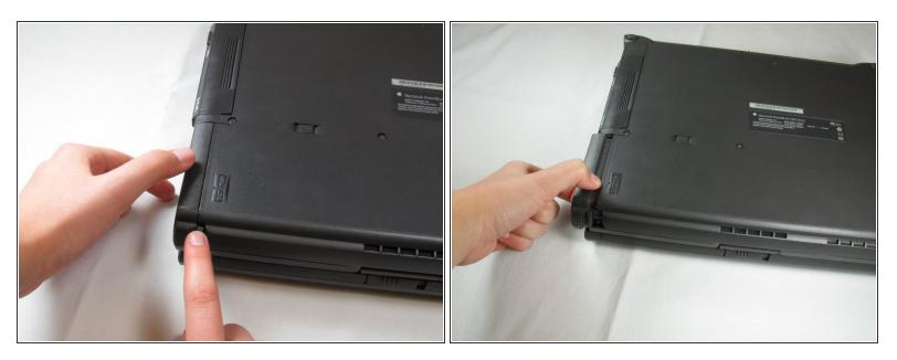
• Hold the button on the front left side and slide the battery out.
