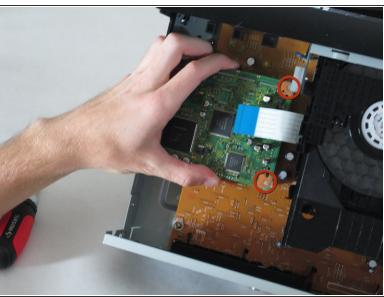
Using tweezers or pliers, squeeze the tabs of the plastic fasteners together. While doing this, gently lift up on the motherboard until the fasteners are released.
