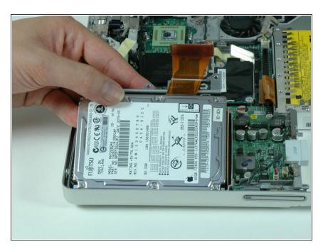
Lift the hard drive up and out of the computer.
