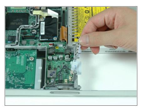
Remove the silver EMI fingers located near the battery contacts.
