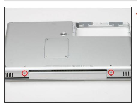
Remove the two Phillips screws from either side of the display hinge.
