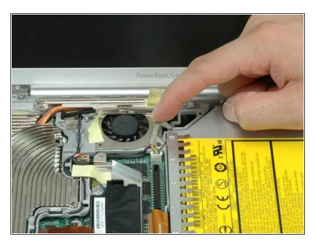
Peel up the Bluetooth cable on the right side of the fan.
