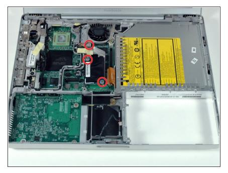
Remove the three Phillips screws securing the modem and modem shield to the logic board.
