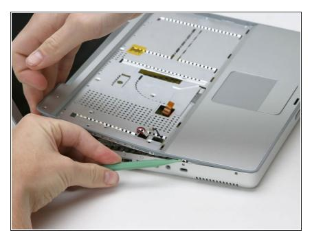
Starting at one of the upper corners near the screen, work around the frame, separating the upper case from the lower case.
