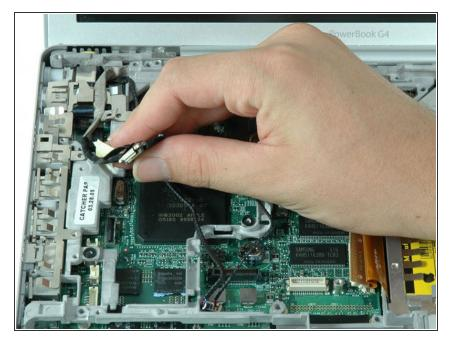
Peel up the yellow tape securing the display data cable to the metal framework, and deroute the display data cable from its slot in the framework.
