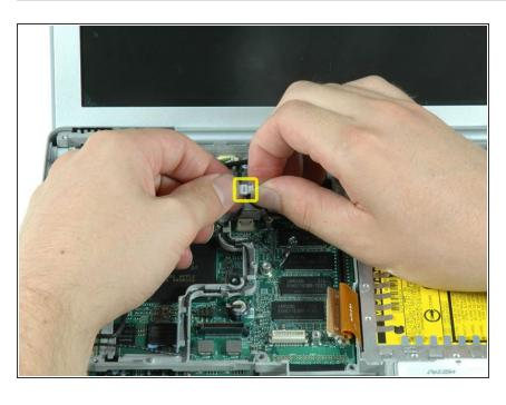
Lift up middle speaker cable from the lower left corner of the fan, and disconnect the two sections of the cable.
