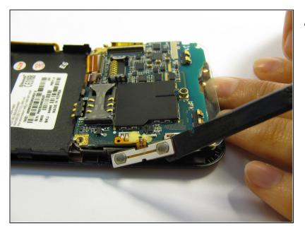
• Peel the button sensor on the side of the motherboard off of the case.
