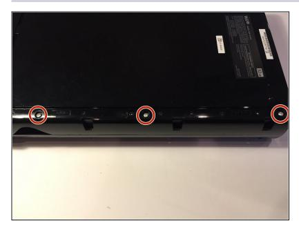
Remove three Tri-Wing screws with a Y1 Tri-Wing screwdriver.
