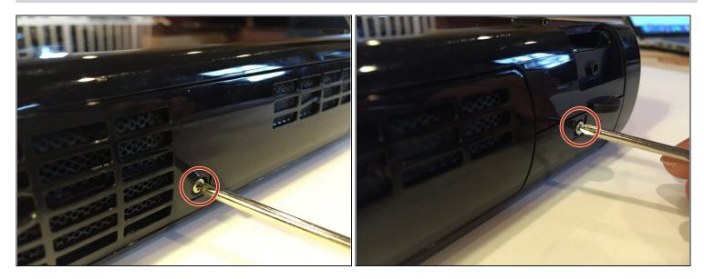
• Unscrew the two screws on the side of the Wii U near the air vents with a Phillips #00 screwdriver.
