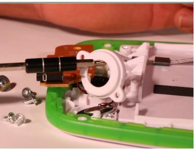
Locate the circular plastic speaker cover, remove the two 5.0mm Phillips screws holding it in place, and gently lift the cover away from the device.
