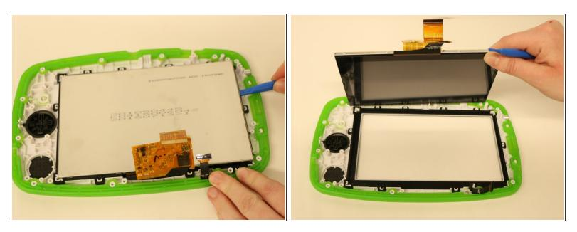
• The screen is now completely accessible and can be lifted out of its cradle. Use the plastic spudger to safely and carefully lift the screen up.
