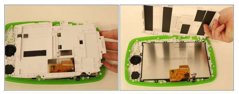
• Carefully lift out the plastic plate and set it aside.
