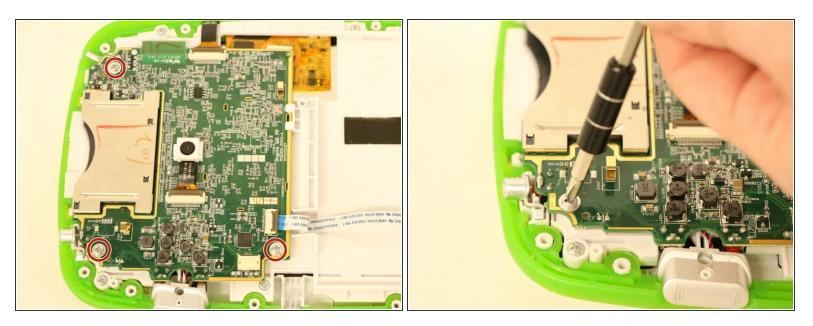
• Remove the three 4.0 mm Phillips screws located in the corners of the motherboard.
