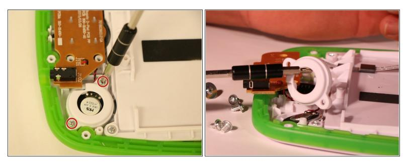
Locate the circular plastic speaker cover, remove the two 5.0mm Phillips screws holding it in place, and gently lift the cover away from the device.
