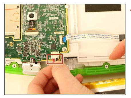
The battery has red, black, and white wires that are all connected to the motherboard through a plastic clip. Unplug this plastic clip to fully remove the battery from your device.
