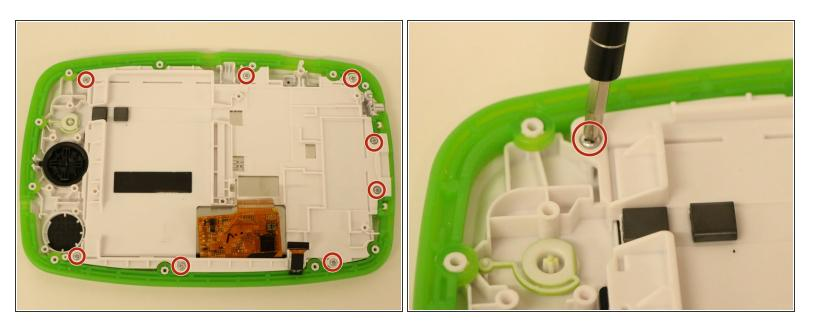
• Remove the eight 4.0 mm screws for the plastic backing that covers the screen.
