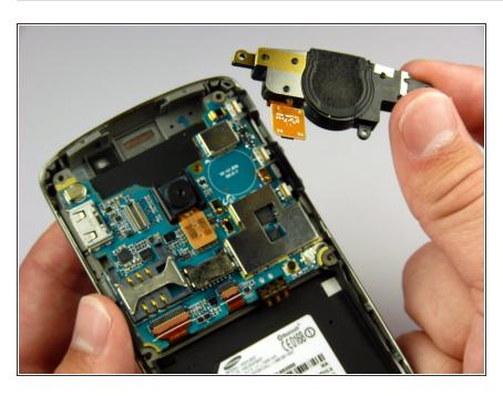
Lift the speaker out of its compartment.
