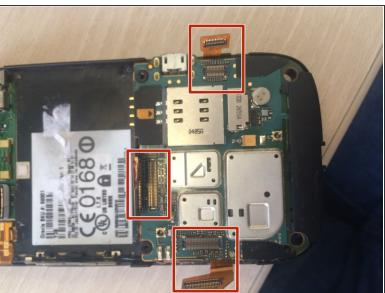
Using your hands, carefully peel the three ribbon cable caps from the logic board.
