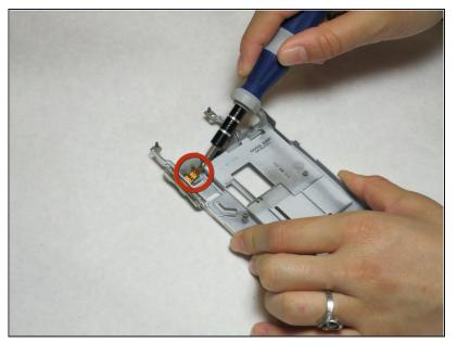
The volume control buttons are secured to the frame only by their fit around a small piece of the plastic. Using a small flat-head screwdriver or other flat object, lift the ribbon over this piece of the cover.
