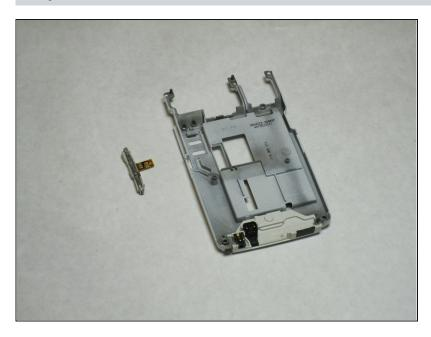
Next, remove the volume control buttons from the cover by pushing or pulling them out away from the interior of the cover.
