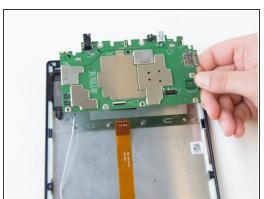
• Lift and pull the motherboard down, gently, towards the case using the tweezers.
