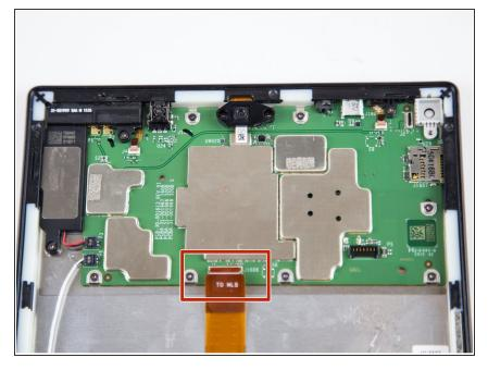
Lift the ZIF connector up to disconnect from the motherboard.
