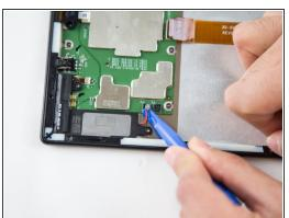
Disconnect the connectors using the plastic opening tool.
