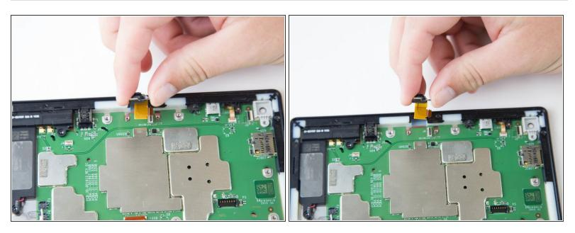
Grip the camera and lift up to detach the ZIF connector from the motherboard.
