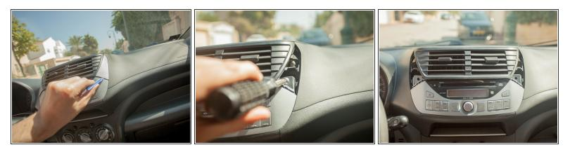
• Use soft disassemble tools to remove the bezels hiding the screws.
