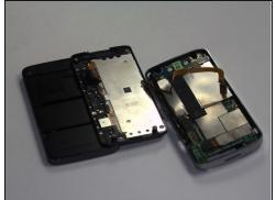
Remove the keyboard ribbon from the motherboard. To do this, simply grasp the ribbon at its base and pry it up at an angle. The ribbon has a metal end that is easily removed from the motherboard.
