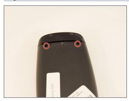
Remove the two 5mm screws located underneath the cover using a J000 Philips screwdriver bit.
