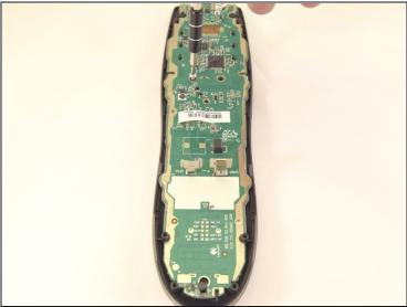
• Using a J0 screwdriver remove the three 5mm screws holding the motherboard to the front face. Two are located just below the processor in the middle of the device and the third is located at the very bottom.
