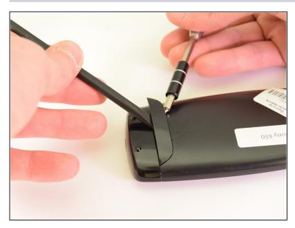
Remove the small plastic cover beneath the plastic LED housing by using a 3.0 flathead screwdriver and a spudger to pry it off. It is glued to the case. If you are having trouble removing it try applying some heat to loosen the glue.
