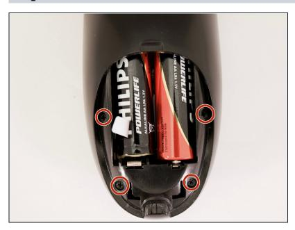
Using a J000 Philips head screwdriver remove the four 5mm screws around the rim of the battery chamber.
