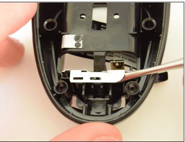
• Using the small end of a spudger, pry out the terminal from the interior of the case.
