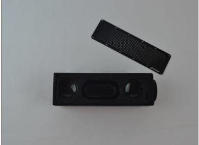
Use a plastic opening tool to pry off the face plate.
