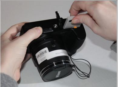
Gently remove the battery from the chamber.
