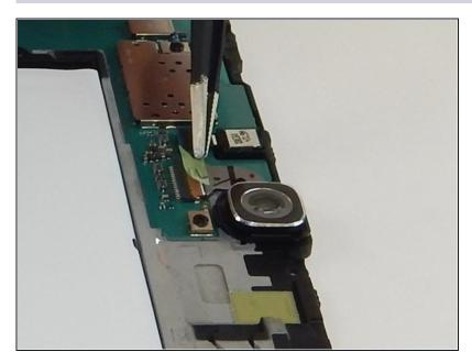
Remove strip of green tape covering the camera connector with the <u>tweezers</u>.
