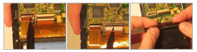
Using tweezers, pull up the other two ZIF connector tabs.
