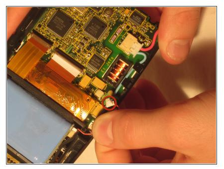
Unhook the battery cable from the motherboard and remove the battery.
