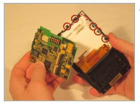
Gently pull the black clips on the inside case to detach the motherboard from the device. Pull the motherboard out towards the bottom left corner.
