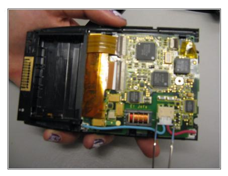
Using tweezers unhook the blue and red screen cables where they connect to the motherboard.
