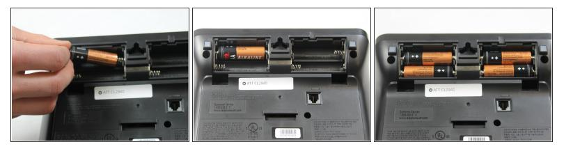
• Place four AA batteries in the battery compartment. Position the negative end (-) at the side with the spring as shown.
