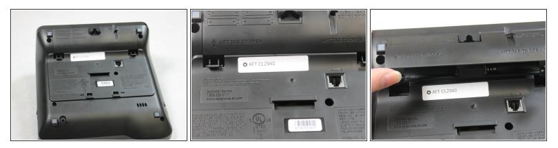
• Flip the phone over and push the tabs upward to release the battery cover.
