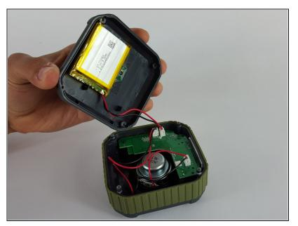
Carefully remove the back cover without breaking the battery wire.
