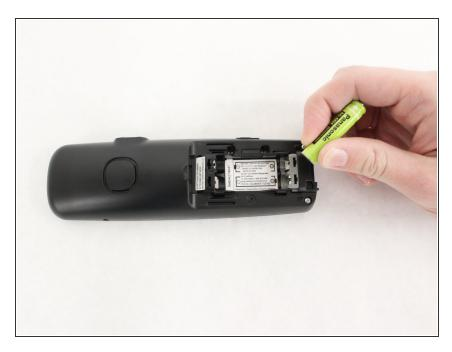
Carefully remove the two batteries by lifting up from one end.
