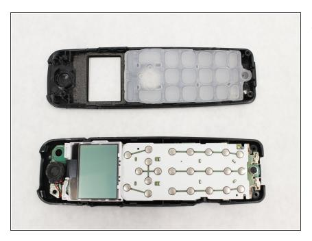
With the screw removed, the front panel assembly can be separated from the rest of the device.
