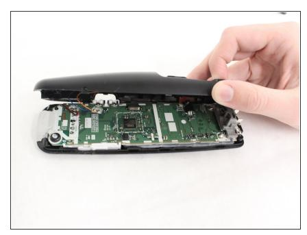
Once the back has been separated from the rest of the device, carefully place it to the side. Be careful not to completely remove it, however, as there are wires connecting the back to the handset.
