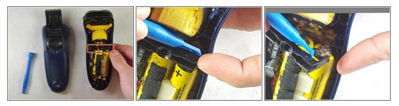
Using the plastic opening tool, carefully pry the inside of the middle bracket towards the outside of the housing in order to remove it.
