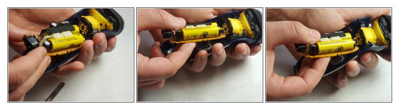
A Cautiously lift and twist the circuit board, then begin sliding the inside assembly forward.
