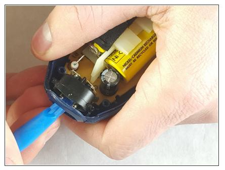
Insert the plastic opening tool into the charging port and push inwards.
