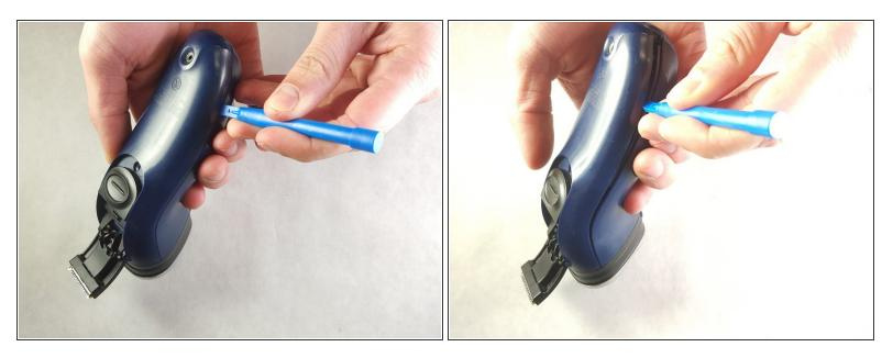
• Separate the back housing and the front housing using the plastic opening tool.
