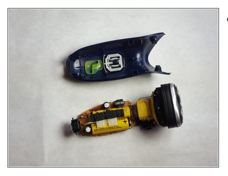
The housing and the inside assembly should be completely separated.
