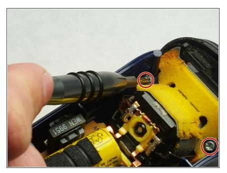
Remove the two T8 2 mm screws near the top of the device shown here.
