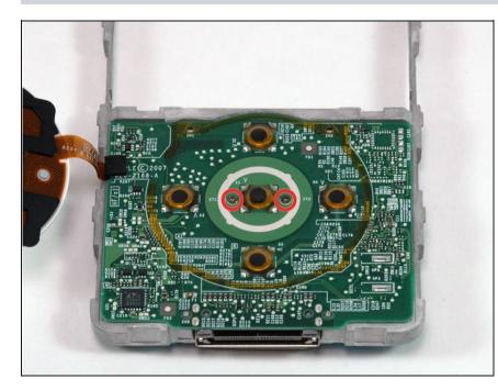
Remove the two Phillips screws securing the logic board to the framework.
