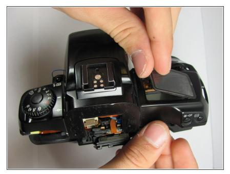
Once the LCD protector has been broken free, lift up on the side adjacent to the flash and pull out the plastic protector. You may now install the new plastic cover.
