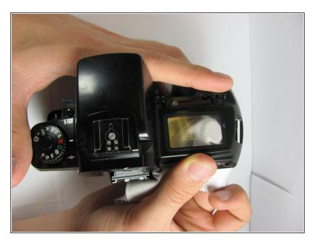
Use a soft cloth to push up on the LCD plastic protector from underneath the top of the camera.
