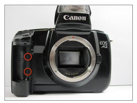
Remove the 5.6mm screws behind the battery cover.
