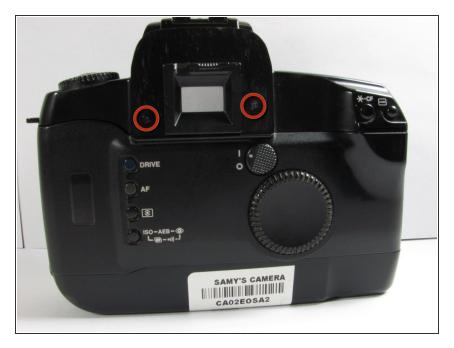
Remove two 4.8mm screws located on both sides of the eyepiece.
