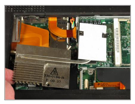
Lift up the heat sink unit from the left side and remove.
