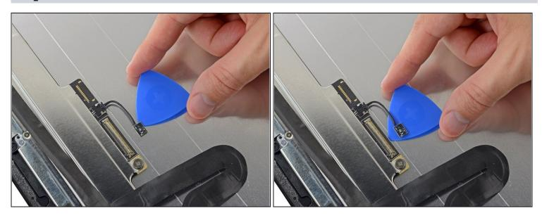
Use an opening pick to break up the adhesive holding the thermal sensor to the back of the iMac display.
