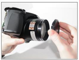
Remove the lens cover to free the zoom motor unit from the camera body.
