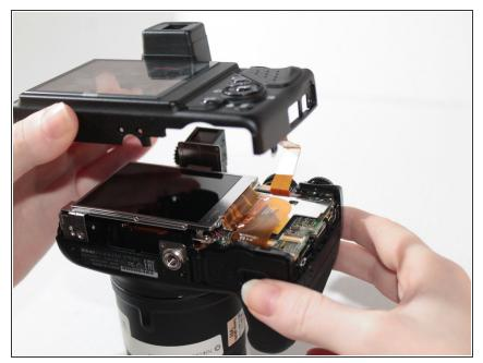
After the ribbon cable is removed from the camera body, the cover can be completely removed.
