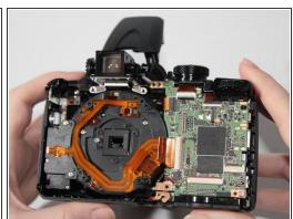
Use the tweezers to remove the CCD sensor carefully.
