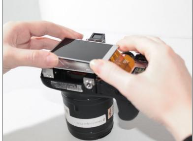
Lift the LCD screen upwards.
