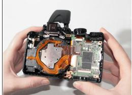
Lift and remove the LCD mounting bracket to expose underlying hardware.
