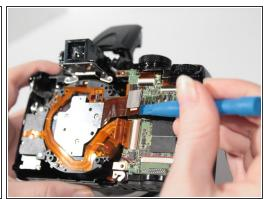
Disconnect the ribbon cable connector by prying upwards on the part using the plastic opening tools.
