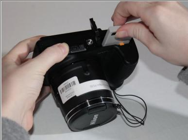
Gently remove the battery from the chamber.
