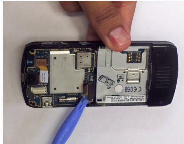
• Using the flat end of the iFixit Opening Tool, carefully disconnect the two connectors from their sockets on the motherboard.
