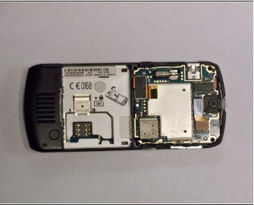
Gently use the iFixit opening tool to lift the metal cover away from the phone.
