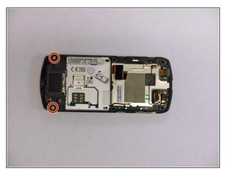
Remove the two T6 screws that are now visible.
